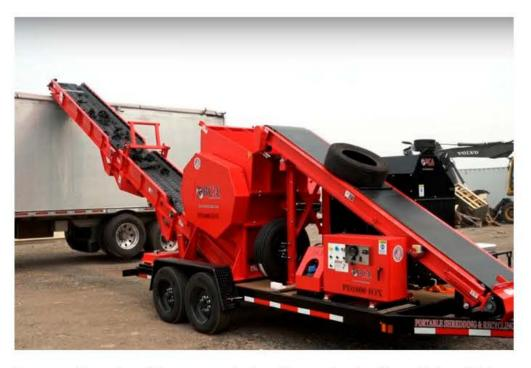
For recyclers shredding tyres, the loading and unloading of shredded materials from conventional scrap containers can be a bottleneck in their operations. Traditional portable shredders cannot reach the height of an open-top walking floor semi-trailer.
